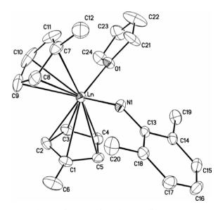
Fig. 1. ORTEP diagram of complexes [Ln = Yb (I), Y (III)] showing atom-numbering scheme. Thermal ellipsoids are drawn at the 30% probability level. Hydrogen atoms are omitted for clarity
